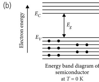
At absolute zero temperature (0 K), the conduction band of a semiconductor is completely empty, *i.e.*,  $\sigma = 0$ . Hence the semiconductor behaves as an insulator. At room temperature, some valence electrons acquire enough thermal energy and jump to the conduction band where they are free to conduct electricity. Thus the semiconductor acquires a small conductivity at room temperature.
