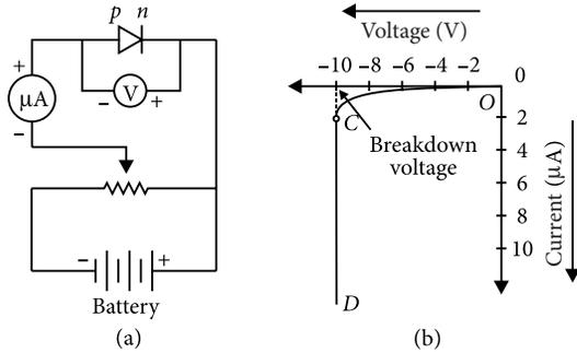
In reverse biased, the applied voltage supports the flow of minority charge carriers across the junction. So, a very small current flows across the junction due to minority charge carriers.
