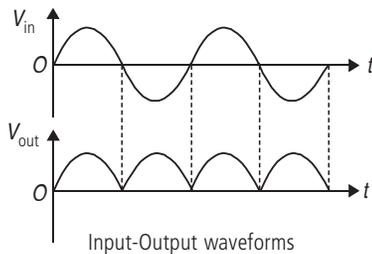
Since in both the half cycles of input a.c., electric current through load  $R_L$  flows in the same direction, so d.c. is obtained across  $R_L$ . Although direction of electric current
