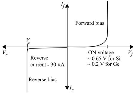
The reverse current is due to minority charge carriers and even a small voltage is sufficient to sweep the minority carriers from one side of the junction to the other side of the junction. Here the current is not limited by the magnitude of the applied voltage but is limited due to the concentration of the minority carrier on either side of the junction.
