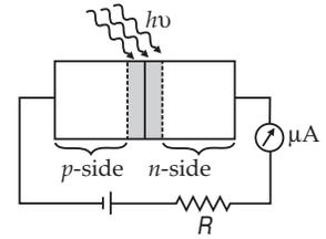
The number of charge carriers increases when light of suitable frequency is made to fall on the  $p-n$  junction, because new electron-hole pairs are created by absorbing the photons of suitable frequency. Intensity of light controls the number of charge carriers. Due to this property photodiodes are used to detect optical signals.
