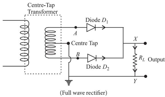
(b) Two  $p-n$  junction diodes can be used to make full wave rectifier which is used to convert alternating current into direct current.
