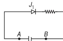
13. In reverse bias condition of photodiode, the change in saturation reverse current is directly proportional to the change in the incident light flux or light intensity, which can be measured accurately. It is not so when photodiode is forward biased.
