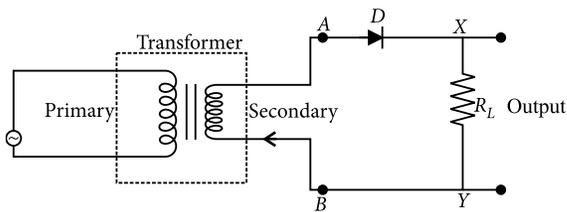
It consists of a diode  $D$  connected in series with load resistor  $R_L$  across the secondary windings of a step-down transformer.
