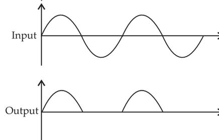
Output frequency of a half wave rectifier = input frequency = 50 Hz
