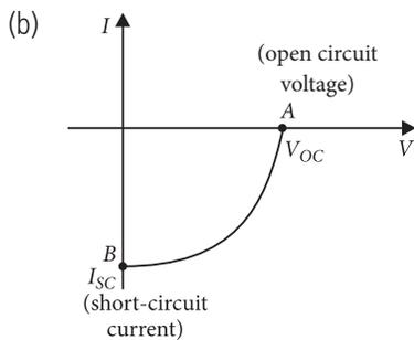
(i)  $V-I$  curve is drawn in the fourth quadrant, because a solar cell does not draw current but supply current to the load.
