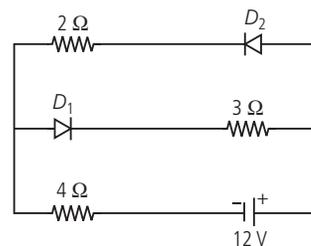
Diode  $D_2$  is forward biased, and offers negligible resistance in the circuit. So current in the branch
