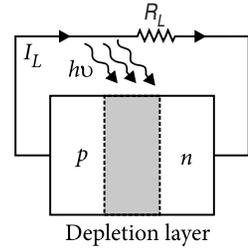
When an external load  $R_L$  is connected as shown in figure, a photocurrent  $I_L$  begins to flow through the load.
