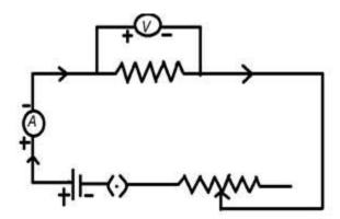
Ohm's law can be proved with the help of the above circuit.
