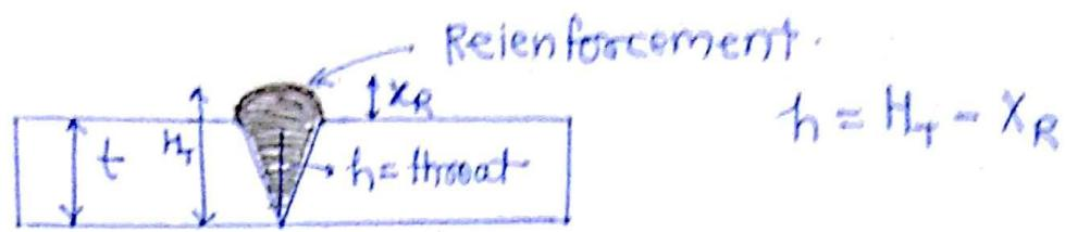
$t < 6 \text{ mm} \rightarrow \parallel \rightarrow \text{square butt weld}$  T
