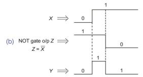
Output Y is logic 1 for small time interval whenever X changes from logic '0' to logic '1', assuming gates are having some delay.
