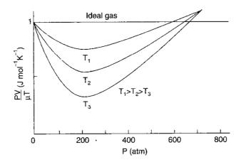
Experimentally value of  $\frac{PV}{\mu T}$  for real gas was calculated by altering the pressure of gas at different
