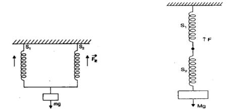
Consider the body of mass M suspended by two springs connected in parallel. Let  $K_1$  and  $K_2$  be the spring constants of two springs.
