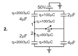
Initial and final charges are marked on 4µf and 2µf capacitors as shown.
