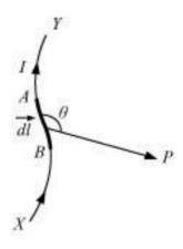
According to this law, the magnetic field is proportional to the current and element length and inversely proportional to the square of the distance.
