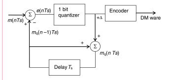
If  $e(nT_s) > 0$ , the o/p quantizer is  $\Delta$  and the o/p of delta modulator is 1.
