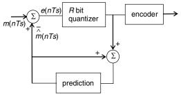
That is, in DPCM, instead of quantizing  $m(nT_s)$  directly, we are quantizing  $e(nT_s) = m(nT_s) - \stackrel{\wedge}{m}$  (nTs).
