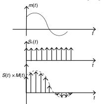
But this kind of instantaneous sampling is very complex to generate. It is possible to construct switches that could operate in an arbitrarily short time. We would never prefer to use them. **Disadvantage:** Crosstalk is more in between the samples.
