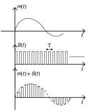
In natural sampling, as in the instantaneous sampling, signal can also be fully recovered by its samples at the receiver side if the sampling has done at Nyquist rate.
