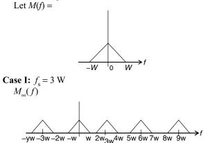
The spectrum of the samples is periodic with period 3 W. At the receiver, if we pass the samples through a low-pass filter of bandwidth W, exactly we can get back M(f) and thus m(t). **Case II:**  $f_s = 2$  W
