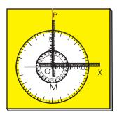
*Fig.4* So,  $sin90^\circ = PM = 1$  and  $cos90^\circ = OM = 0$ .
