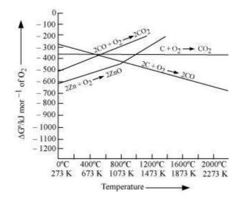
Reduction of ZnO to Zn is usually carried out at 1673 K. From the above figure, it can be observed that above 1073 K, the Gibbs free energy of formation of CO from C and above 1273 K, the Gibbs free energy of formation of  $CO_2$  from C is lesser than the Gibbs free energy of formation of  $ZnO_2$ . Therefore, C can easily reduce ZnO to Zn.
