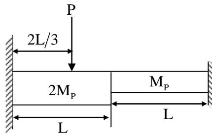
The minimum value of load ( $P$ ) at which the beam would collapse (ultimate load) is
