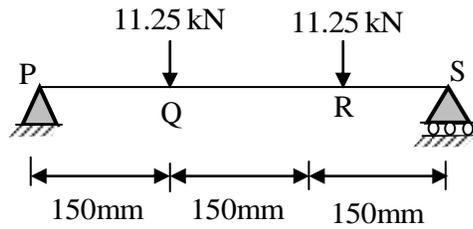
Cross section of the prism is given as 150 mm × 150 mm. Considering linear stress distribution across the cross-section, the modulus of rupture (expressed in MPa) is\_\_\_\_\_.
