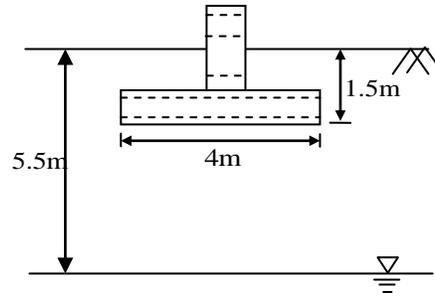
Using Terzaghi's bearing capacity equation and a factor of safety  $F_s = 2.5$ , the net safe bearing capacity (expressed in  $\text{kN/m}^2$ ) for local shear failure of the soil is \_\_\_\_\_.
