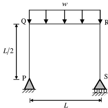
The bending moment in the beam at the joint 'Q' is
