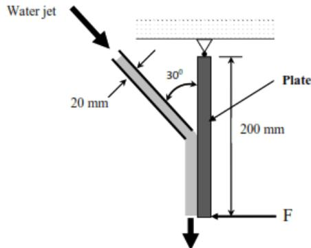
Consider  $g$  as  $9.81 \text{ m/s}^2$  and neglect the self-weight of the plate. The force  $F$  (expressed in N) required to keep the plate in its vertical position is \_\_\_\_\_.
