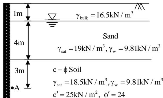
The water table is found 1 m below the ground level. The entire soil mass is retained by a concrete retaining wall and is in the active state. The back of the wall is smooth and vertical. The total active earth pressure (expressed in  $\text{kN/m}^2$ ) at point A as per Rankine's theory is \_\_\_\_\_.
