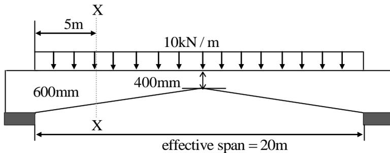
The beam is subjected to a uniformly distributed factored load of intensity 10 kN/m. The design shear force (expressed in kN) at the section X-X of the beam is \_\_\_\_\_.
