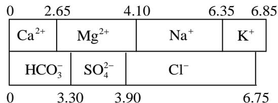
The non-carbonate hardness (expressed in mg/L as CaCO<sub>3</sub>) of the sample is \_\_\_\_\_.
