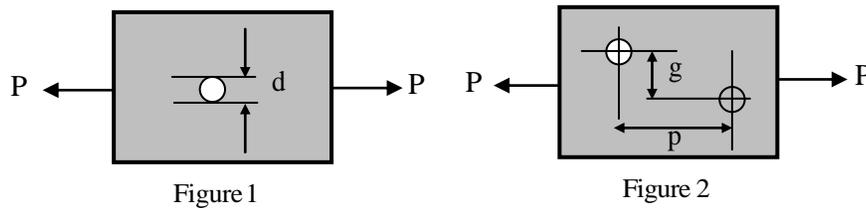
Which one of the following conditions must be ensured to have higher net tensile capacity of configuration shown in Figure 2 than that shown in Figure 1?
