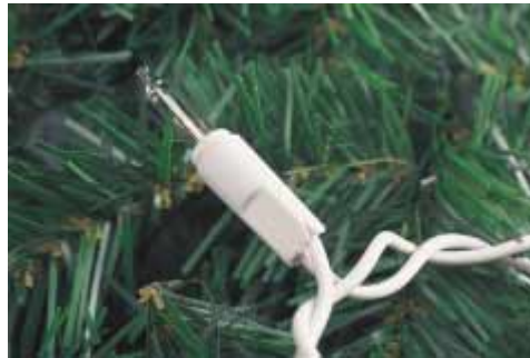
Figure 28.10 (a) Schematic diagram of a modern “miniature” holiday lightbulb, with a jumper connection to provide a current path if the filament breaks. (b) A Christmas-tree lightbulb.
