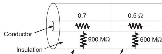
$$(R_{eq})_{conductor} = 0.7 + 0.5 = 1.2 \Omega$$
