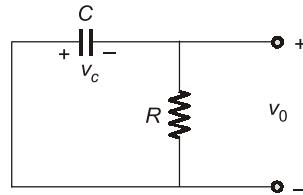
$$v_c(t) = V_{c\max} \left( \frac{T}{2} \right) e^{-t(T/2)\tau}$$
