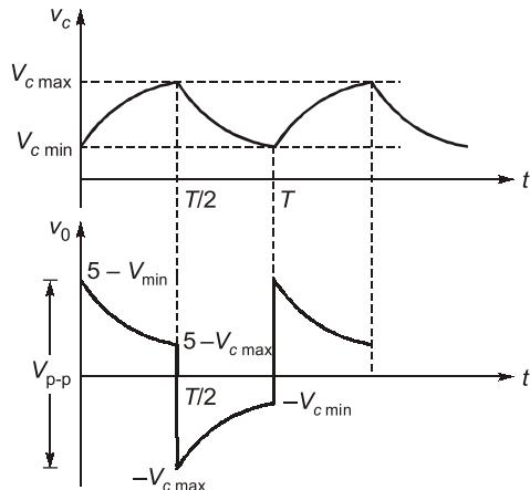
$$\text{For 1st half cycle, } V_0 = V_i - V_c$$
