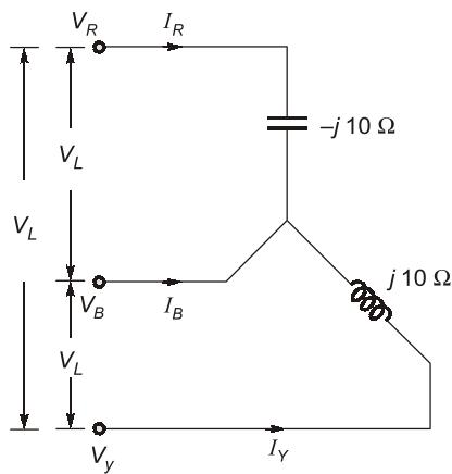
$$I_R = \frac{V_{RB}}{-j10} = \frac{V_L \angle -60^\circ}{-j10} = \frac{V_L}{10} \angle 30^\circ$$
