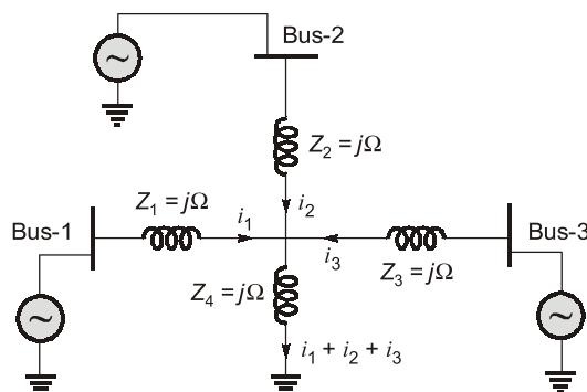
$$V_1 = j1i_1 + j1(i_1 + i_2 + i_3)$$
