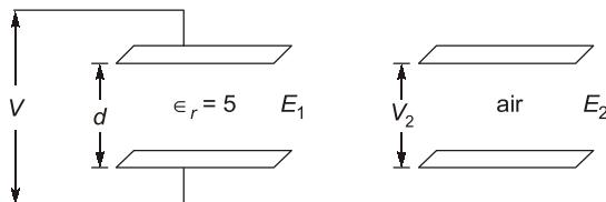
If voltage source is removed then in both cases charge  $Q$  is constant.
