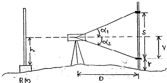
$$\text{RL of } Q = \text{RL of BM} + h - V - r$$
