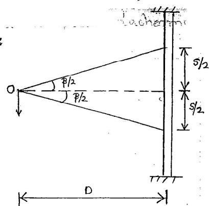
$$D = \frac{s}{2 \times \left(\frac{\beta}{2}\right)} = \frac{s}{\beta} \times 206265 ; \beta \text{ in seconds}$$
