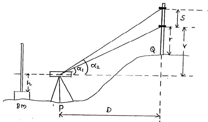
$$\text{RL of } Q = \text{RL of BM} + h + v - r.$$
