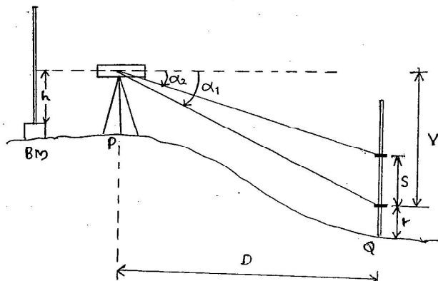
$$\text{RL of } Q = \text{RL of BM} + h - v - r$$
