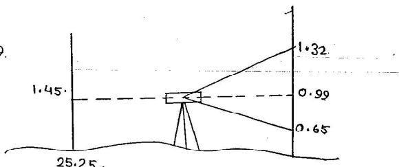
$$\begin{aligned} Q.3 \quad D &= ks \cos^2 \theta + c \cos \theta \quad \left\{ \text{if not given, assume } k=100 \right\} \\ &= 100 (2.985 - 2.225) \cos^2 (7^\circ 54') = \underline{\underline{74.564}} \text{ m} \end{aligned}$$
