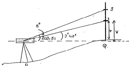
$$RL \text{ of } Q = 203.51 + 2.535 - 1 = \underline{\underline{205.045}} \text{ m}$$
