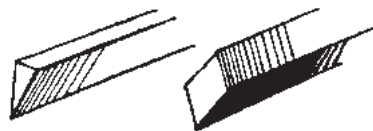
Pointed burin for copper engraving
