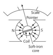
Its working is based on the fact that when a current carrying coil is placed in a magnetic field, it experiences a torque. This torque tends to rotate the coil about its axis of suspension in such a way that the magnetic flux passing through the coil is maximum.
