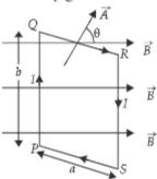
Force on side PQ or RS of loop is  $F = IbB \sin 90^\circ = Ib B$  and perpendicular distance between two non-collinear forces is  $r_{\perp} = a \sin \theta$
