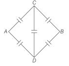
The circuit is a balanced bridge. We can remove the capacitor between C and D.
