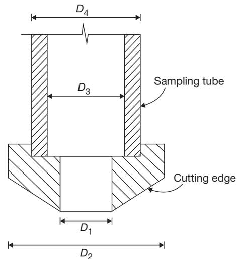
For obtaining good quality undisturbed samples, the area ratio should be 10 percent or less.
