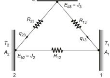
$$q_{23} = \frac{E_{b2} - E_{b3}}{R_{23}} = \frac{\sigma(T_2^4 - T_3^4)}{\frac{5}{\pi D^2}}$$
