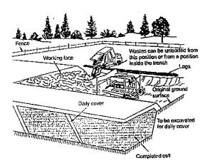
Fig. 6.4 Trench method of landfilling solid wastes for small landfills.
