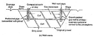
Flg. 6.5 Typical methods for venting landfill gases: (a) cell; (b) trench; (c) well
