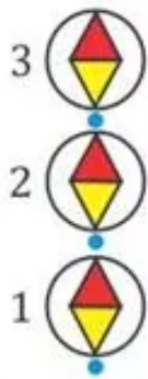
(a) Plotting a field line with a compass needle
