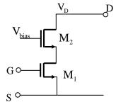
The circuit is used as amplifier with the input connected between G and S terminals and the output taken between D and S terminals.  $V_{bias}$  and  $V_{D}$  are so adjusted that both transistors are in saturation. The transconductance of this combination is defined as  $g_{m} = \frac{\partial i_{D}}{\partial v_{GS}}$  while the output resistance is  $r_{0} = \frac{\partial v_{DS}}{\partial i_{D}}$ ,
