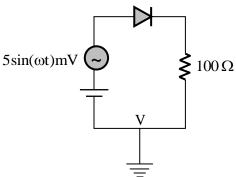
For  $\omega = 2 \times 10^6$  rad/s, the amplitude of the small-signal component of diode current (in  $\mu A$ , correct to one decimal place) is \_\_\_\_\_.
