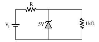
Assume that the Zener diode has a constant reverse breakdown voltage for a current range, starting from a minimum required Zener current,  $I_{Z(min)} = 2mA$  to its maximum allowable current.
