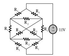
The magnitude of the current (in amperes, accurate to two decimal places) through the source is \_\_\_\_\_.
