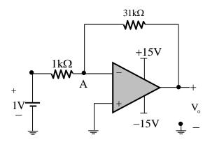
In the above circuit, assume the op-amp to be ideal. The voltage (in volts, correct to one decimal place) at node A, connected to the negative input of the op-amp as indicated in the figure is\_\_\_\_\_\_.
