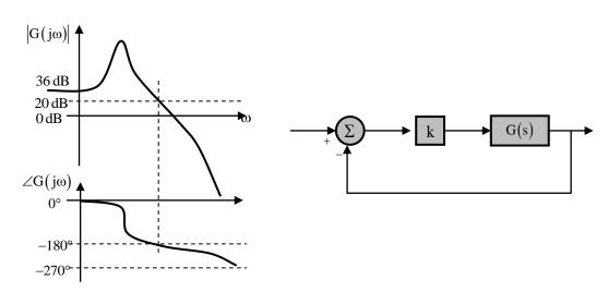
Consider the negative unity feedback configuration with gain k in the feedforward path. The closed loop is stable for  $k < k_0$ . The maximum value of  $k_0$  is \_\_\_\_\_\_.
