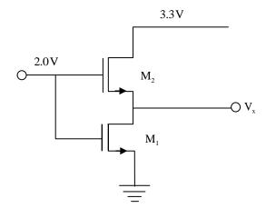
Note that  $V_{GS}$  for  $M_2$  must be > 1.0 V.
