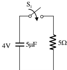
The charge (in  $\mu\text{C}$ ) lost by the capacitor from  $t = 25\mu\text{s}$  to  $t = 100\mu\text{s}$  is \_\_\_\_\_.
