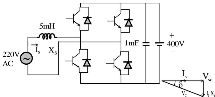
All devices are ideal. It is used to charge a battery at 400V with power of 5kW from a source sinusoidal AC mains at unity p.f. If its ac side interfacing inductor is 5mH and the switches are operated at 20kHz, then the phase shift ( $\delta$ ) between AC mains voltage ( $V_s$ ) and fundamental AC rms VSC voltage ( $V_{Cl}$ ), in degree, is\_\_\_\_\_.
