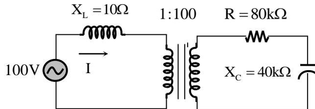
The applied primary voltage is 100V (rms), 50Hz, AC. The rms value of the current I, in ampere, is \_\_\_\_\_.
