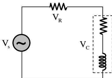
The rms values of possible voltage across the resistance ( $V_R$ ) and coil ( $V_C$ ) respectively, in volts, are
