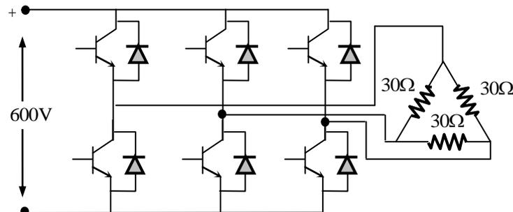
If it is fed from a 600V battery, with  $180^\circ$  conduction of solid-state devices, the power consumed by the load, in kW, is \_\_\_\_\_.
