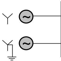
Both the generators are having positive, negative and zero sequence impedance of  $j0.4$  p.u.,  $j 0.3$  p.u and  $j0.15$  p.u., respectively. If the pre-fault voltage is 1 p.u., for a line-to-ground (L-G) fault at the terminals of the generators, the fault current, in p.u., is \_\_\_\_\_.
