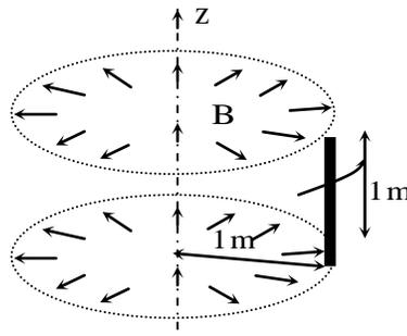
The speed of the conductor in r.p.m. required to induce a voltage of 1V across it, should be \_\_\_\_\_.
