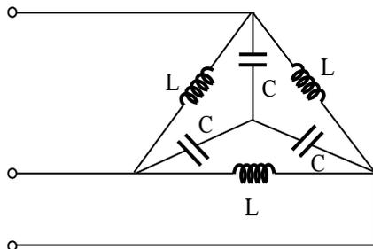
The value of the capacitance (C) for which all the line currents are zero, in millifarads, is \_\_\_\_\_.
