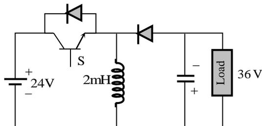
It is operated at 20kHz with an inductor of 2 mH and output capacitor of 1000  $\mu\text{F}$ . All devices are considered to be ideal. The peak voltage across the solid-state switch (S), in volt, is \_\_\_\_\_.
