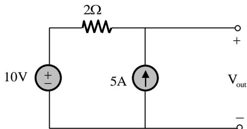
The voltage ( $V_{out}$ ) across the current source, in volts, is
