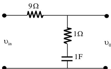
the frequency (in rad/s) at which the maximum phase lag occurs is \_\_\_\_\_.
