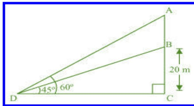
Let BC be the building, AB be the transmission tower, and D be the point on the ground from where the elevation angles are to be measured.
