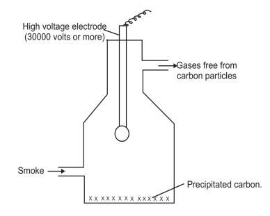
Fig.8.8 : Cottrell smoke precipitator
