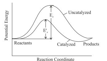
Fig. 15.8 : Graphical representation of the effect of catalyst on a reaction.
