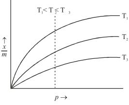
Fig. 17.5 : Adsorption isotherm of a gas
