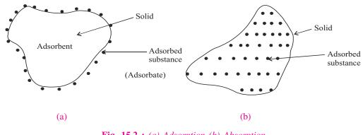
Fig. 15.2 : (a) Adsorption (b) Absorption
