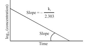
Fig. 14.1 : A graph of log<sub>10</sub> (concentration) against time for a first-order reaction.
