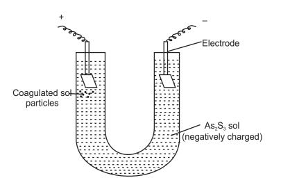
**Fig. 8.7 :** *A set up for Electrophoresis*
