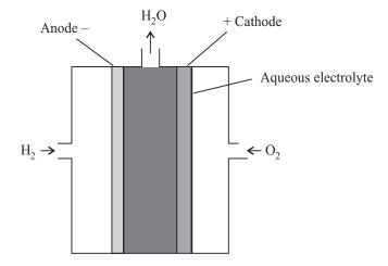
Figure 13.12: Hydrogen-oxygen fuel cell
