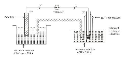
**Fig. 13.9** : Measurement of standard electrode potential of Zn/Zn<sup>2+</sup> electrode
