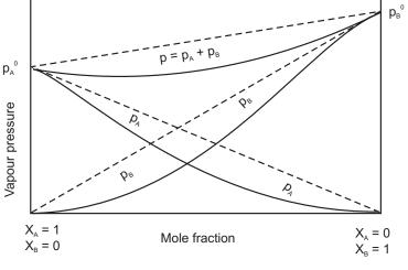
Fig. 7.4 : Negative deviation for a liquid pair
