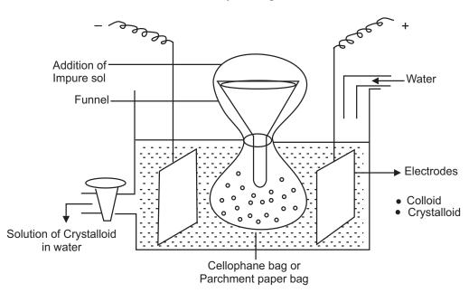
Fig. 8.4 : Electrodialysis
