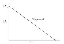
Fig. Concentration versus time plot for a zero order reaction.
