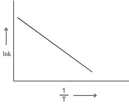
**Fig. 14.3** Graphical determination of  $E_{a}$ .
