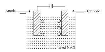
Fig. 13.4 : Electrolytic cell
