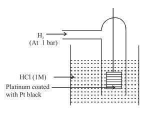
Fig. 13.8 : Standard Hydrogen electode
