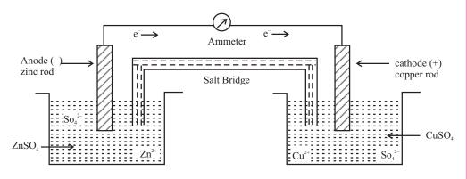
Fig. 13.6 : Daniell cell having zinc and copper electrodes
