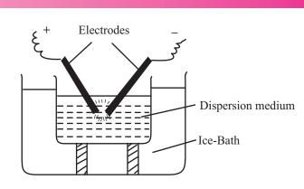
Fig. 8.2 : Preparation of colloidal solution by Bredig's Arc Method
