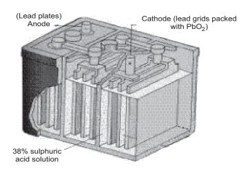
Fig. 13.11: Lead storage battery
