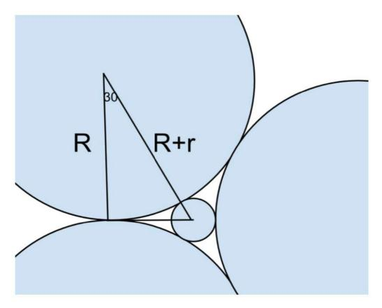
Using this right angle triangle, we can get the relation:  $\frac{R}{R+r}=\frac{\sqrt{3}}{2}$  We can take  $R=\sqrt{3}a$  and R+r as 2a, this would give us r as  $R=\left(2-\sqrt{3}\right)a$
