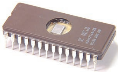
Figure 3.7 Erasable Programmable Read Only Memory
