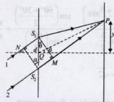
Path difference between ray 1 and 2 reaching  $P = NS_1 + S_1M$  $\Delta x_1 = d \sin \alpha + d \sin \theta$
