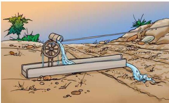
Fig. 1.4 (b) : Chain pump
