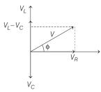
Phasor diagram for *L-C-R* series circuit for  $X_L > X_C$
