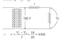
**22** For the case of DC, the frequency is zero and the net impedance is equal to the resistance. For the case of AC, the impedance of the AC circuit is given by  $Z = \sqrt{R^2 + \omega^2 L^2}$
