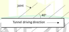
Dip of the joint:  $20^{\circ} - 45^{\circ}$
