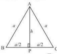
Area of an equilateral  $\Delta = \frac{1}{2} \times a \times \frac{\sqrt{3}}{2} a = \frac{\sqrt{3}}{4} a^2$ , where a is the length of its one side
