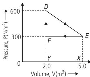
$$\text{Work done in complete cycle} = \text{Area of } \Delta DEF = \frac{1}{2} \times EF \times DF \\ = \frac{1}{2} \times 3 \times 300 = 450 \text{ J}$$
