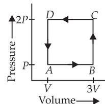
**30. (b):** Work done during cyclic process *ABCD* = area enclosed by *ABCD*
