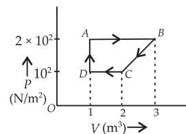
**31. (d):** In going from *B* to *C* and from *D* to *A*,  $V = \text{constant}$ . So,  $\Delta V = 0$ .
