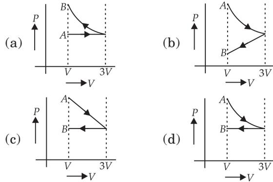
36. The  $P$ - $V$  diagram of path followed by one mole of perfect gas in a cylindrical container is shown in figure, the work done when the gas is taken from state  $A$  to state  $B$  is
