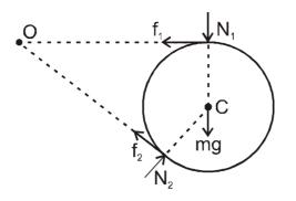
Net torque on rod about hinge 'O' = 0
