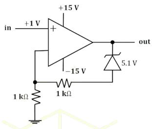
**Solution: Step 1:** In the given op-amp circuit, the Zener diode is in the feedback loop with a breakdown voltage of 5.1 V. The Zener diode operates in the breakdown region, which means the voltage across it will be clamped to 5.1 V, regardless of the output voltage of the op-amp. **Step 2:** The op-amp operates in the linear region, and the voltage across the Zener diode remains constant at 5.1 V. The input voltage is +1 V, and since the op-amp is configured in a
