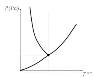
(A) Clausius-Clapeyron equation is valid across the melting curve and the vaporization curve
