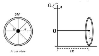
**Solution: Step 1:** The total moment of inertia of the wheel is the sum of the moments of inertia of the rim and the point mass at the center.
