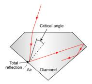
The total internal reflection of light is used in diamond polishing to create a gleaming brilliance. It is adjusted by polishing the diamond with specific cuts so that the majority of light rays approaching the surface are incident with an angle of incidence greater than the critical angle. As a result, they are subjected to multiple reflections and eventually emerge from the top of the diamond. This gives the diamond a brilliant gleam.
