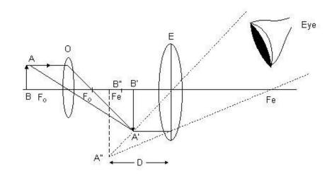
Here, O = objective lens E = Eye piece AB = object, A" B" = final image Magnifying power (*m*) of a compound microscope is given by
