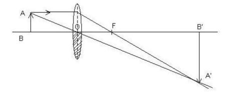
For the given case, there will be no change in height of image as we can see in ray diagram above although it will be less bright.
