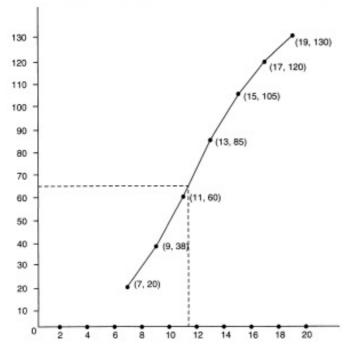
This curve is the required cumulative frequency curve or an ogive of the less than type.
