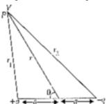
Two point charges q and -q are located at points (0, 0,- a) and (0, 0, a) respectively.
