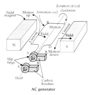
Principle: It is based on the principle of electromagnetic induction. That is, when a coil is rotated about an axis perpendicular to the direction of the uniform magnetic field, an induced emf is produced across it.
