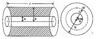
Consider an elementary cylindrical shell of radius r and thickness dr. Its area of cross section (normal to flow of current) =  $2\pi r l$  and its length = dr.
