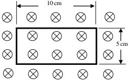
The plane of the loop is perpendicular to the field lines. The resistance of the loop is  $0.4\Omega$ , and its inductance is negligible. The magnetic flux density (in Tesla) is a function of time, and is given by B(t) = 0.25 sin  $\omega$ t, where  $\omega = 2\pi \times 50$  radian/second. The power absorbed (in Watt) by the loop from the magnetic field is \_\_\_\_\_
