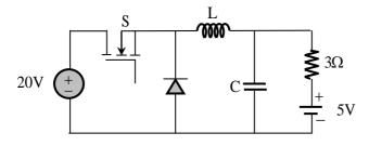
If the inductor and capacitor are sufficiently large to ensure continuous inductor current and ripple free capacitor voltage, the charging current (in Ampere) of the 5 V battery, under steady-state, is
