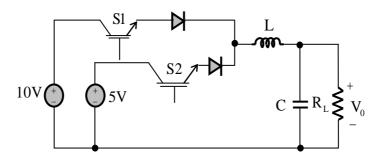
Assuming continuous conduction of the inductor current and negligible ripple on the capacitor voltage, the output voltage  $V_0$  (in Volt) across  $R_L$  is \_\_\_\_\_\_.
