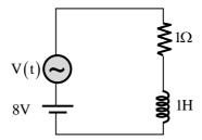
The instantaneous voltage of the AC source (in Volt) is given by v(t) = 12sint. If the circuit is in already state, then the rms value of the current (in Ampere) flowing in the circuit is \_\_\_\_\_.
