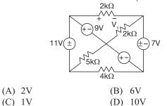
6. The value of  $i_x$  in the given figure is \_\_\_\_\_ Amp.
