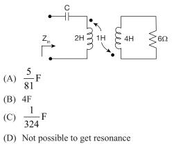
**28.** The circuit shown in below figure, if the current through inductor  $L_2$  is Zero Then Which one of the following relation is correct
