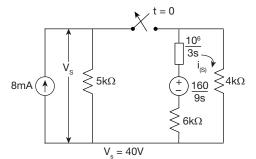
Capacitor will discharge through 6 k $\Omega$  and 4 k $\Omega$  resistors  $I_c = -i_R$ Applying KVL
