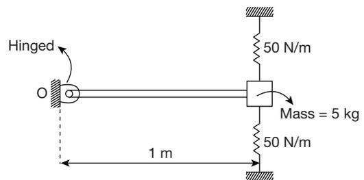
Assuming  $EI$  of rod = 2.67 N-m<sup>2</sup>, calculate natural frequency of the bar in (rad/sec)
