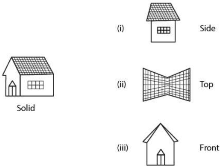
4. For each of the given solid, the three views are given. Identify for each solid the corresponding top, front and side views.
