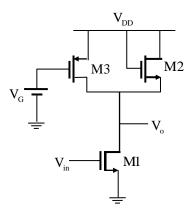
Also, all transistors operate in saturation and have negligible body effect. The ac small signal voltage gain  $(V_0/V_{in})$  of the circuit is
