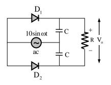
Assuming that the diodes do not breakdown in the reverse bias, the output voltage V<sub>0</sub> (in volt) at the steady state is \_\_\_\_\_.
