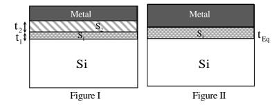
The capacitor in Figure II has only insulator material X of thickness  $t_{Eq}$ . If the capacitors are of equal capacitance, then the value of  $t_{Eq}$  (in nm) is \_\_\_\_\_.
