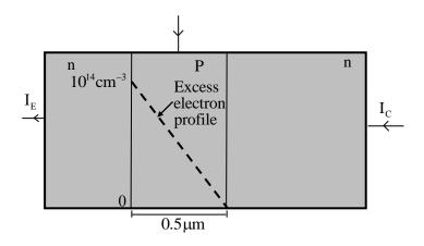
If the area of the emitter-base junction is 0.001 cm<sup>2</sup>,  $\mu_n = 800 \text{ cm}^2/(V-s)$  in the base region and depletion layer widths are negligible, then the collector current I<sub>c</sub> (in mA) at room temperature is
