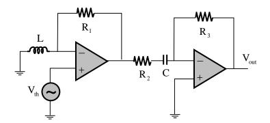
If the input  $V_{in} = \cos(10^6 t)$ , then the overall voltage gain  $(V_{out}/V_{in})$  of the circuit is \_\_\_\_\_. Answer: (-1)
