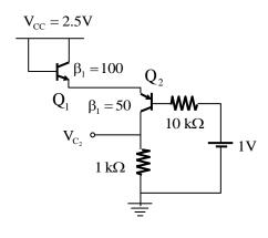
Assuming  $V_{BE1} = V_{EB2} = 0.7$  volt, the value of the dc voltage  $V_{C_2}$  (in volt) is \_\_\_\_\_.
