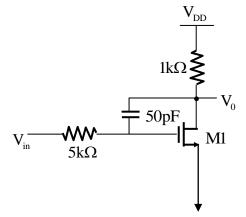
Ignoring internal parasitic capacitances and assuming the channel length modulation  $\lambda$  to be zero, the small signal input pole frequency (in kHz) is \_\_\_\_\_.
