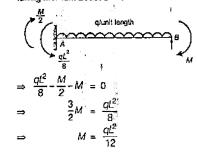
(c) (Ef)<sub>b</sub> → ∞, means beam will not bend any more because its flexural rigidity is infinite so, column AB will behave as the column shown in figure below
