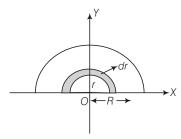
(a) The half-disc can be supposed to be consists of a large number of semicircular rings of mass dm and thickness dr and radii ranging from r = 0 to r = R.
