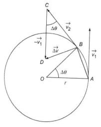
Consider a body of mass m moving along a circular path of radius r. A and B denote the position of the body at times t and  $(t + \Delta t)$  and the angular displacement is  $\Delta \theta$  in time  $\Delta t$ .
