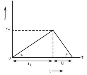
Slope of v-t graph = acceleration Therefore,  $\alpha = \frac{v_m}{t_1}$ ,  $\beta = \frac{v_m}{t_2}$   $\frac{1}{\alpha} = \frac{t_1}{v_m}$ ,  $\frac{1}{\beta} = \frac{t_2}{v_m}$   $\frac{1}{\alpha} + \frac{1}{\beta} = \frac{t_1 + t_2}{v_m} = \frac{\alpha + \beta}{\alpha\beta}$  $v_m = \frac{(t_1 + t_2)\alpha\beta}{\alpha + \beta} = \frac{\alpha\beta T}{\alpha + \beta}$
