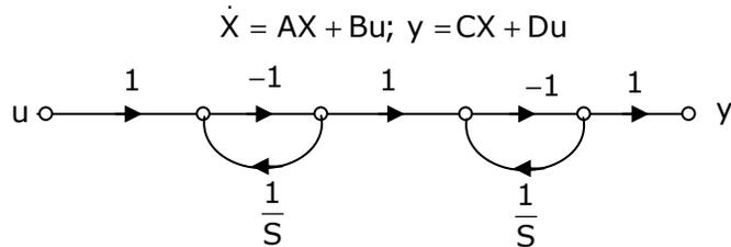
54. The state-variable equations of the system shown in the figure above are
