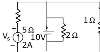
50. The current  $I_S$  in Amps in the voltage source, and voltage  $V_S$  in Volts across the current source respectively, are
