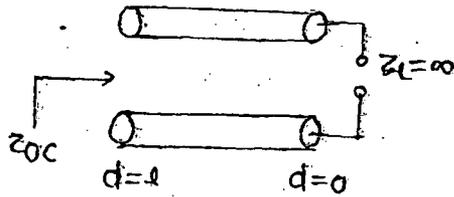
$$Z(d=l) = \frac{Z_0 (Z_L + Z_0 \tanh(\gamma l))}{Z_0 + Z_L \tanh(\gamma l)}$$
