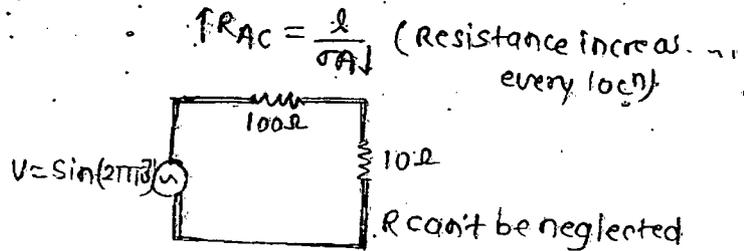
(i)  $R \rightarrow$  Whenever high freq. signal flowing through a cond<sup>r</sup> cross sectional area decreases, so that resistance comes in to the picture of every location.
