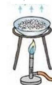
Crystallization- pure crystals of solid separate out on cooling saturated solution (copper sulphate)
