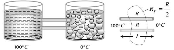
$\frac{Q}{t} = \frac{(\theta_1 - \theta_2)}{R} \Rightarrow \left(\frac{Q}{t}\right)_1 = \frac{mL}{t} = q_1 L = \frac{(100-0)}{\frac{R}{2}} \dots (i)$
