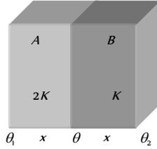
$$\Rightarrow \frac{4}{3} \frac{KA \times 60}{2x} = \frac{2K \cdot A \times (\Delta\theta)_A}{x} \Rightarrow (\Delta\theta)_A = 20K$$
