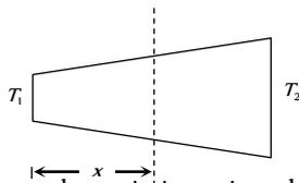
Material of the conductor is isotropic and its curved surface is thermally isolated from surrounding. Its ends are maintained at temperatures  $T_1$  and  $T_2$  ( $T_1 > T_2$ ). If, in steady state, heat flow rate is equal to  $H$ , then which of the following graphs is correct
