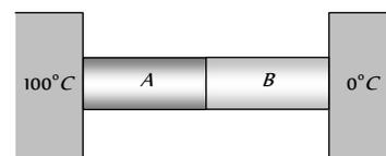
63. A cylindrical rod having temperature  $T_1$  and  $T_2$  at its ends. The rate of flow of heat is  $Q_1\text{ cal/sec}$ . If all the linear dimensions are doubled keeping temperature constant then rate of flow of heat  $Q_2$  will be
