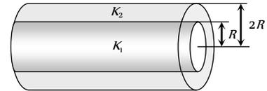
Hence  $K_{eq} = \frac{K_1 A_1 + K_2 A_2}{A_1 + A_2}$ ; where  $A_1$  = Area of cross-section of inner cylinder =  $\pi R^2$  and  $A_2$  = Area of cross-section of cylindrical shell =  $\pi \{ (2R)^2 - (R)^2 \} = 3\pi R^2$
