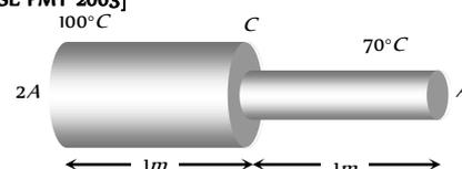
67. The ratio of the coefficient of thermal conductivity of two different materials is 5 : 3. If the thermal resistance of the rod of same
