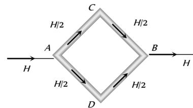
Heat current will flow from A to B via path ACB and ADB. Since all the rods are identical so  $(\Delta\theta)_c = (\Delta\theta)_d$ .
