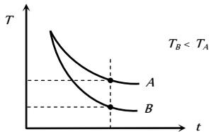
It is clear that, at a particular time after start cooling, temperature of oil will be less than that of water.
