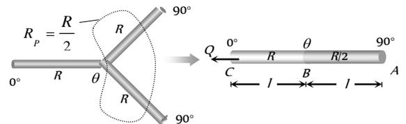
$$\therefore \frac{Q}{t} = \frac{(\theta_1 - \theta_2)}{R} \text{ and } \left( \frac{Q}{t} \right)_{AB} = \left( \frac{Q}{t} \right)_{BC}$$
